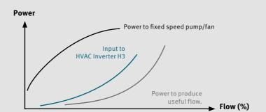
Using HVAC Inverter H3 compared to direct on line control, an estimated 20% reduction in speed results in potential energy savings of 50%.
